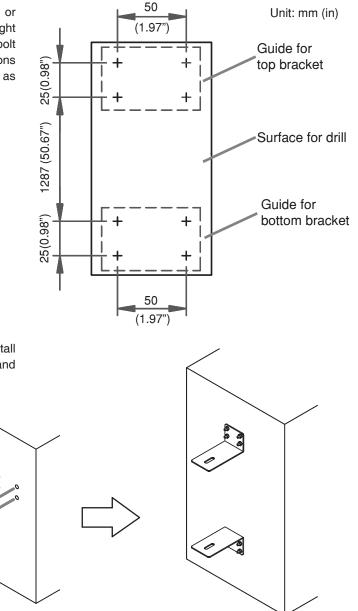
Step 2. Drill the surface that have been marked, install the proper dyna bolt then the both of top and bottom bracket.
